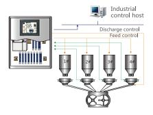
Multi-material serial weighing and networking
