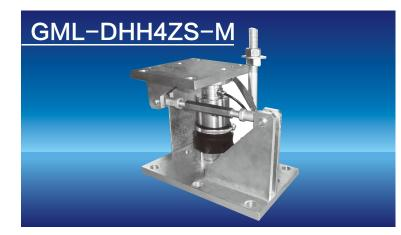
Equipped with self-restoring rocker pin load cell GML-DHH4ZS, Accuracy class C2,C3 .
