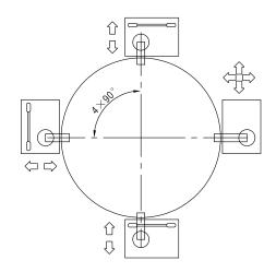
Rectangular arrangement of the weighing module below tanks
