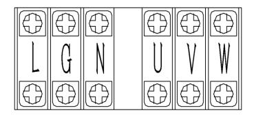
Figure 2-4 Power supply and motor interface diagram
