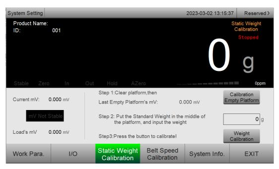
Figure 3-11 shows an example of the weight calibration interface Description of static calibration parameters:
