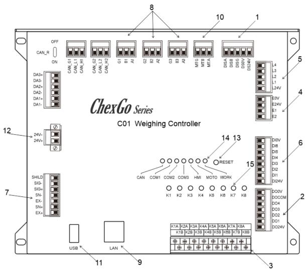
Figure 2-2 Control panel of weighing scale
