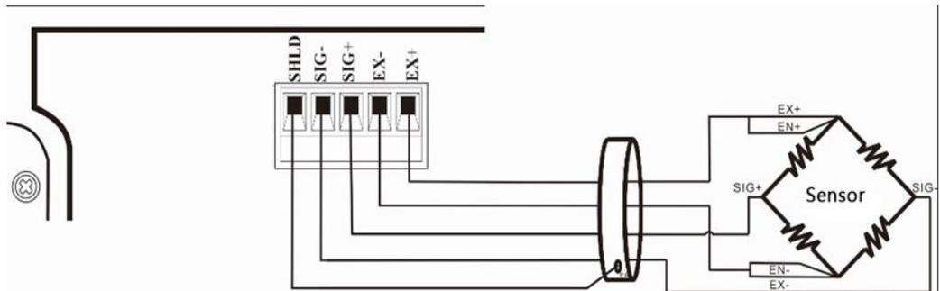
**EX+**: Power supply positive    **EX-**: power supply negative    **SN+**: induction positive
