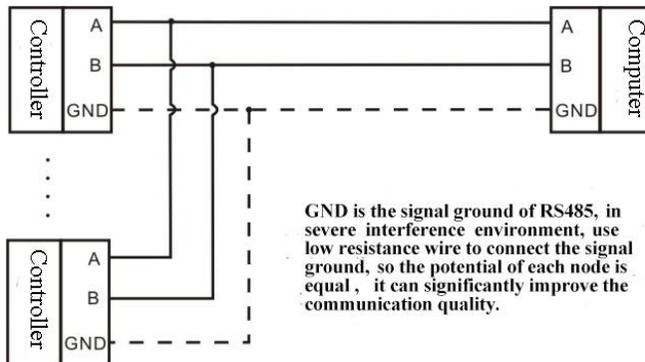
Connection diagram between instrument and upper computer (RS-485 mode)
