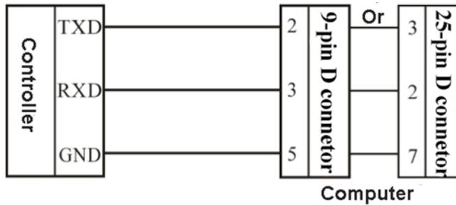
Meter to computer connection diagram (RS-232 mode)
