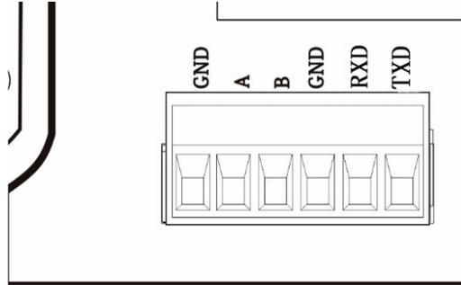
Meter and computer connection diagram:
