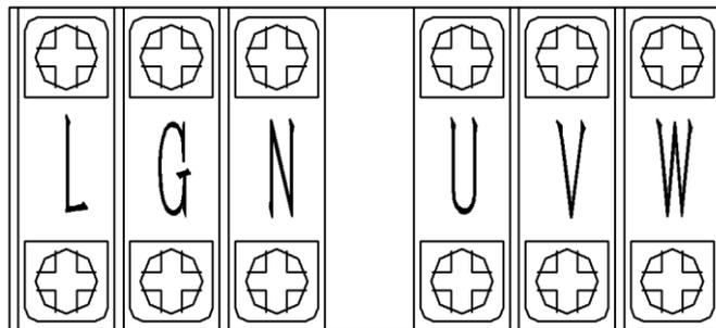
Figure 2-4 Power supply and motor interface diagram
