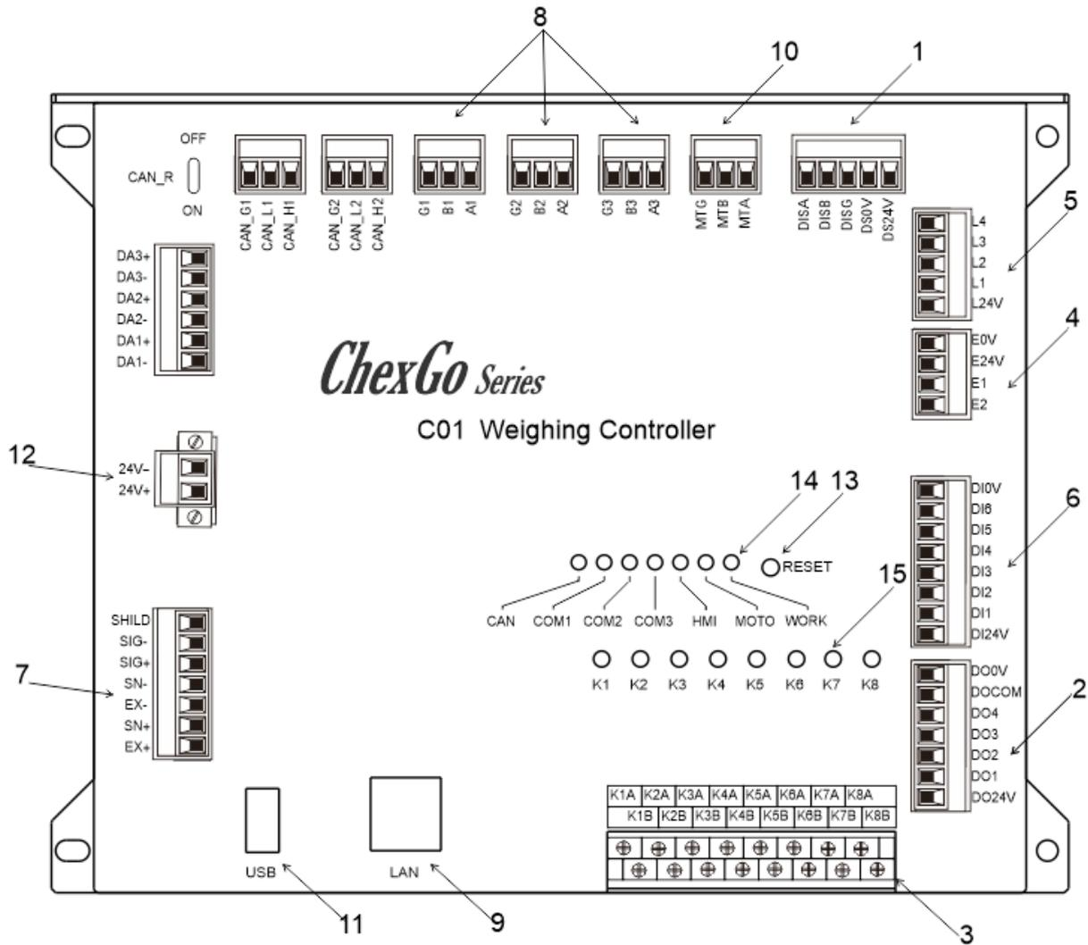
Figure 2-2 Control panel of weighing scale
