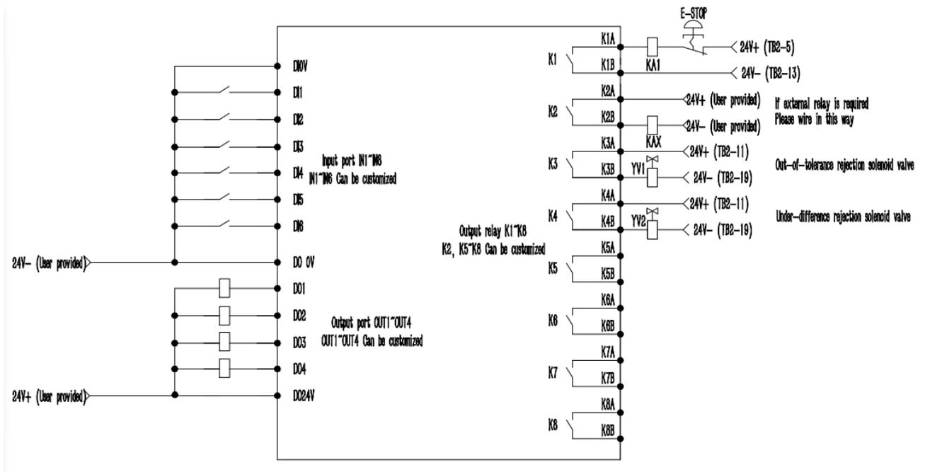
Figure 2-3 Schematic diagram of inlet and outlet connections
