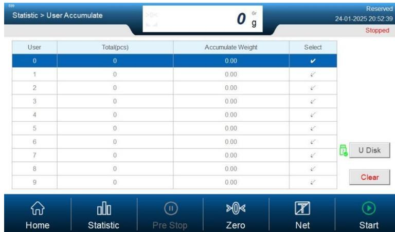
The User accumulation interface allows you to select the corresponding user data for export to a USB drive, and it can also be manually cleared.
