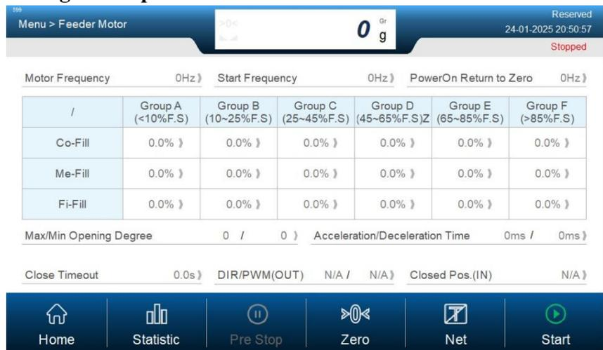
The parameters of this interface are set by factory default and no modification is required; The interface involves motor frequency, starting frequency and power-on return-to-zero frequency And the percentage opening angle of the motor for coarse feed、 medium feed、 fine feed. Maximum opening degree, minimum opening degree, acceleration time, deceleration time. Close gate timeout, motor direction and pulse output, close gate in place input.
