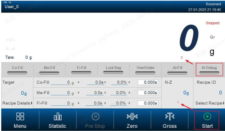
When the weighing is completed, the AI Debugging text will change to Debugged, and at the same time, the AI-fill status indicator light will light on and enter the intelligent feeding status, then the device can work normally and can enter the history record to view the data of each batches.
