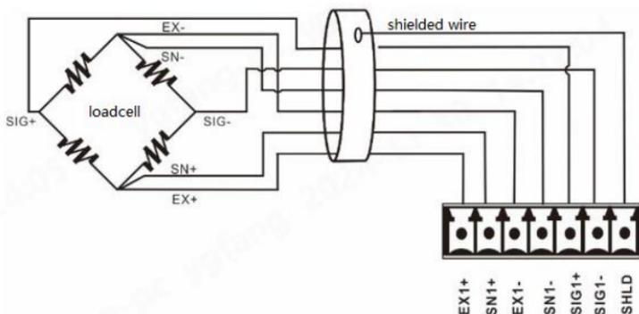
Four-wire connection (using loadcell 1 as an example) :
