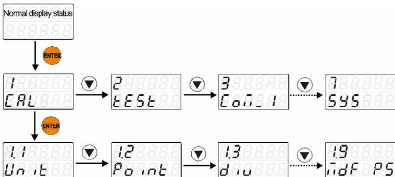
1). Press Keys  $\blacktriangledown$   $\blacktriangle$  to select the required items before the same level, taking 1 CAL standard parameter as an example, that is, when 1.1 unit is displayed, Press the key  $\blacktriangledown$  can be switched to 1.2 point, and press the key  $\blacktriangle$  can be switched to 1.9 mdf ps.
