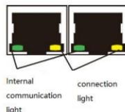
**Connection light:** The network cable is connected properly and the connection light is blinking.
