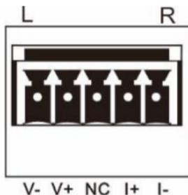
voltage output; **V-**: Negative voltage output
