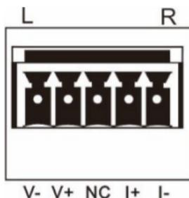
voltage output; **V-**: Negative voltage output
